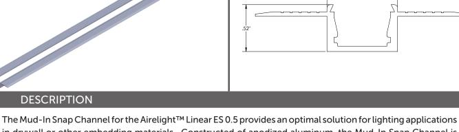
in drywall or other embedding materials. Constructed of anodized aluminum, the Mud-In Snap Channel is low profile and light weight providing ultimate flexibility for the lighting designer. Once mounted into the selected building material, the attachment clips on the Airelight<sup>™</sup> ES model simply snap into the channel, providing easy integration and a secure attachment.
