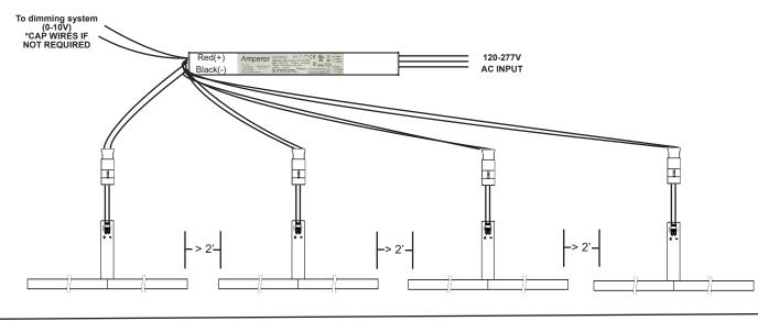
Wiring Example #2: Airelight Linear2 0.5s mounted end to end (less than 2' end to end)
