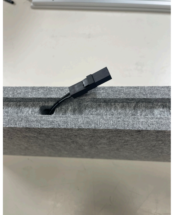
4) Remove mating male connector from input connector adjacent to hanging hardware.
